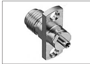
Two-hole panel-mounted jack for 0.047-inch semi-rigid cable FLA-H-SPF16BG+
